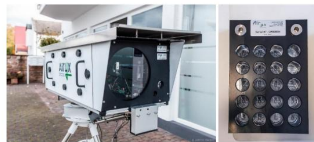
Left: Telescope unit of the AiryX Open Path system. Right: Retro reflector array.
